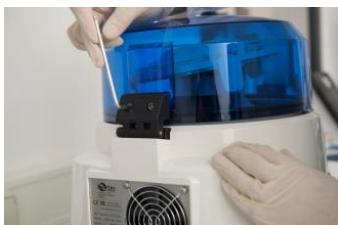
2. Place the new lid on the Precellys® Evolution without the cooling module
