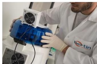
3. Insert the reinforced hinge over the Precellys® hinge and screw it to the lid
